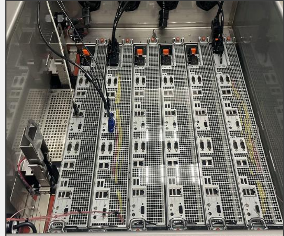
12U 15KW immersion liquid cooling tank Fluid: Synthetic Oil (PAO Family)
