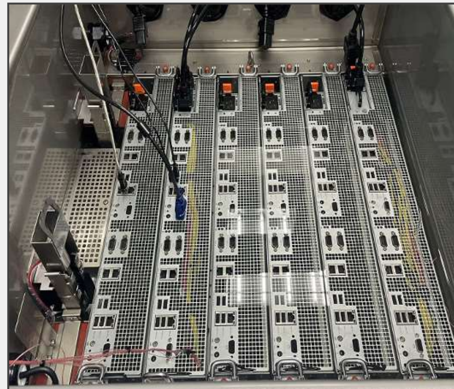
12U 15KW immersion liquid cooling tank Fluid: Synthetic Oil (PAO Family)
